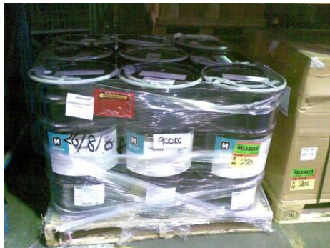
✓ Stabilised load well labelled
