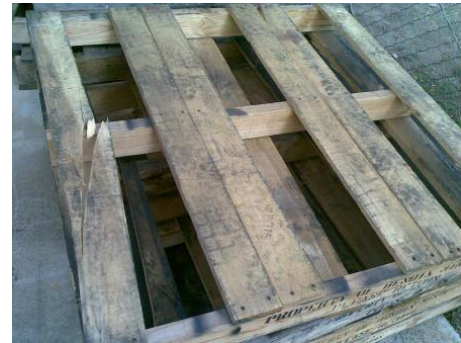
X Cracked planks
