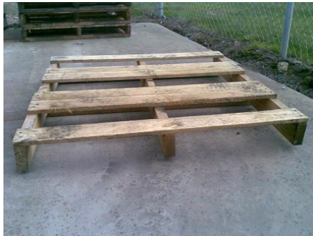
X Missing planks
